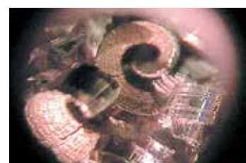
1刃3.5mmの切粉 Chip from One Edge, 3.5mm
